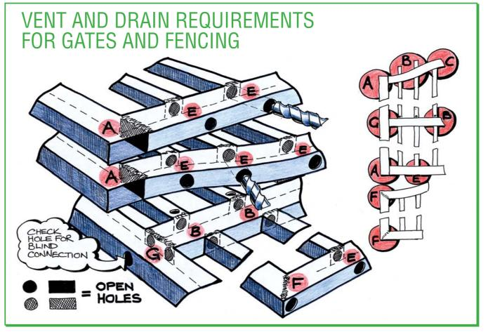
Vessels and hollow sections, including those in small diameter tubular fabrications, MUST be vented to atmosphere for the safety of galvanizing personnel and to prevent possible damage to the article. At galvanizing temperatures, moisture trapped in closed sections is converted rapidly to superheated steam, generating explosive forces unless vented.
