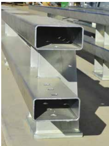
Figure 1: With a specified minimum HDG coating thickness of 85μm, AS/NZS 2312.2 can be used to estimate this bridge rail will be protected from rust for over 50 years in a C3 (medium) environment.
